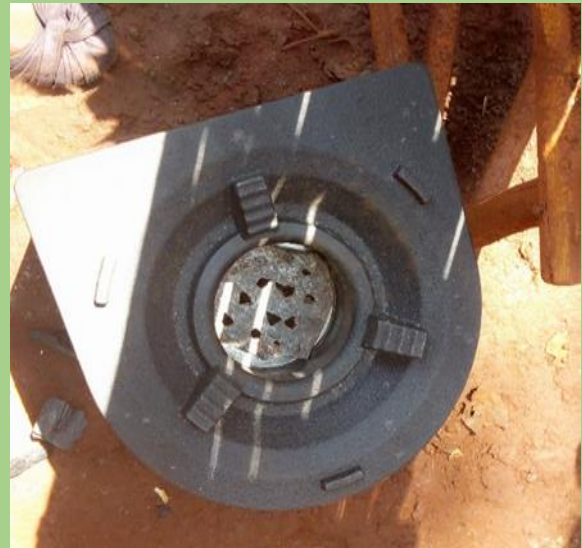
Photo 29: Demonstration of insert stove for the artisan who implemented repairing of insert stove.
