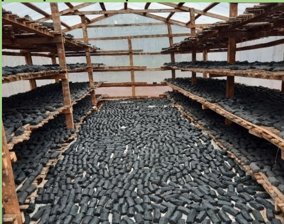
Photo 44: Depicting produced Briquettes inside the drying parlour in Nduta Camp.
