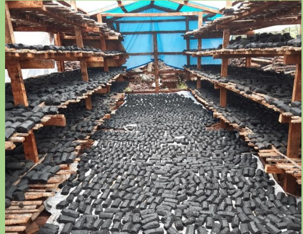
Photo 45: Representing produced briquettes inside drying parlour which is open to one end.
