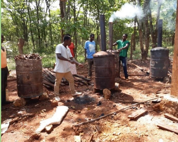
Photo 39: Charring process taking place by using metal kiln.
