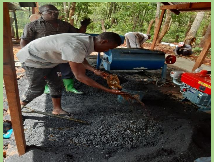
Photo 42: Incentive worker rationing between charred materials and molasses binders.
